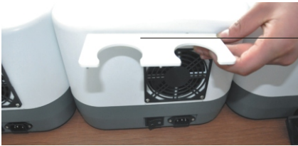
Fix the probe Holder by screw
